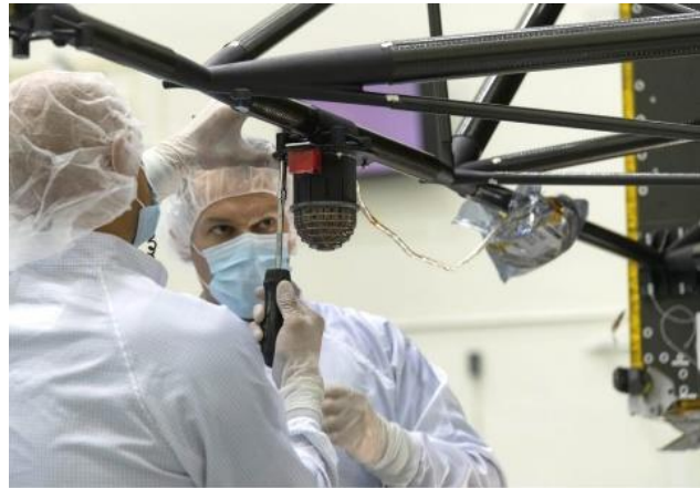
Abbildung 5: Psyches Magnetometer. © NASA/JPL-Caltech.
